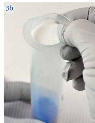
4. Insert the DLV plunger into the disposable cartridge.
