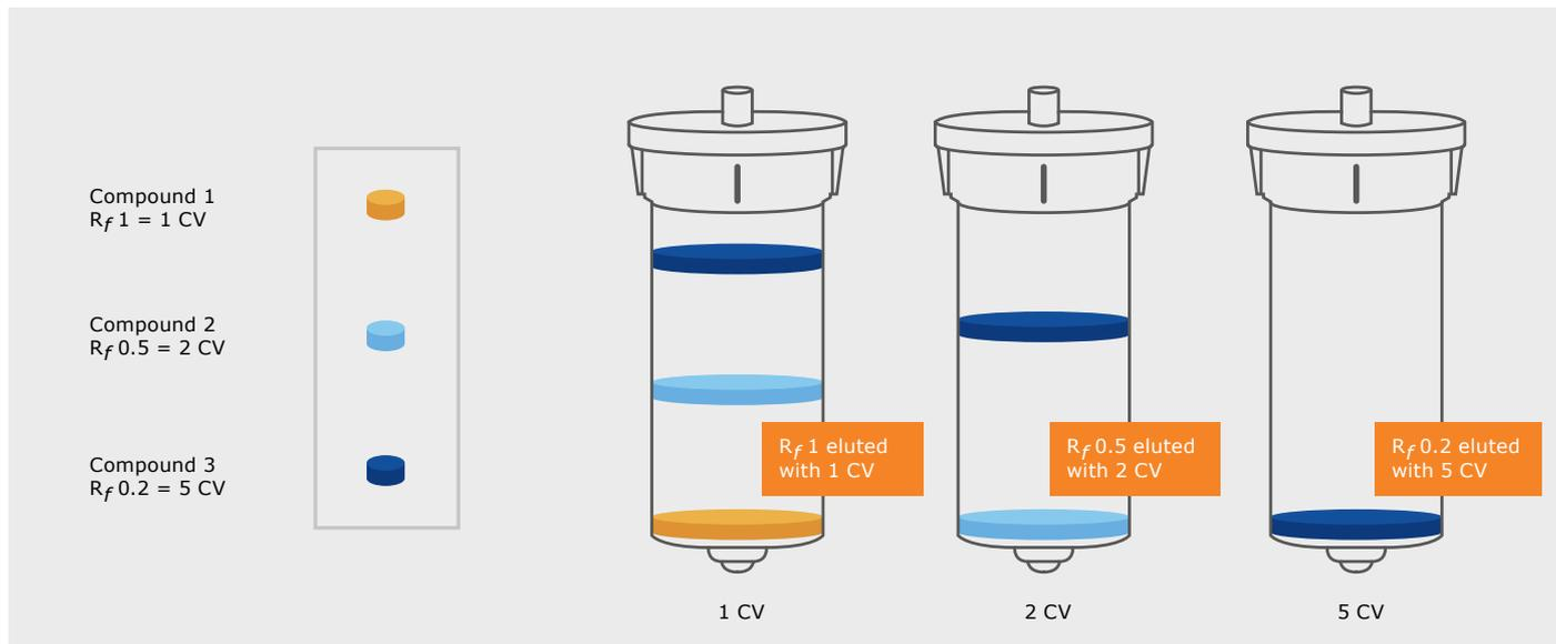
Figure 11. Conversion from TLC to Column Chromatography. Compound 1 has an  $R_f$  of 1, and since  $Cv=1/R_f$  the a single column volume of solvent is all that is needed to elute Compound 1. Compound 2 has an  $R_f$  of 0.5 and since  $CV=1/0.5 = 2$ , Compound 2 will elute in two column volumes. Finally Compound 3 has an  $R_f$  of 0.2 resulting in a CV of 5 meaning that it will take 5 column volumes of solvent to elute Compound 3.
