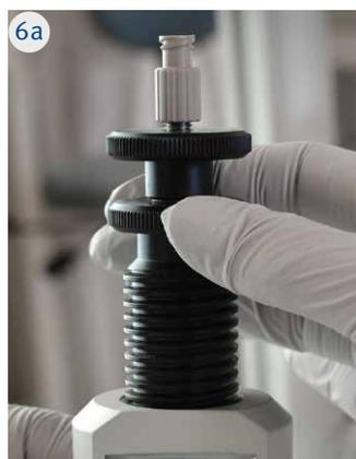
7. Turn the upper nut on the plunger clockwise to lock the o-ring. Finger-tighten.
