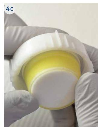
5. Insert the cap with Samplet® into the cartridge top and tighten firmly. Ensure the cap is even and fully tightened down, there should be no more than a 1 mm gap between the cap and the mounting fin as shown.
