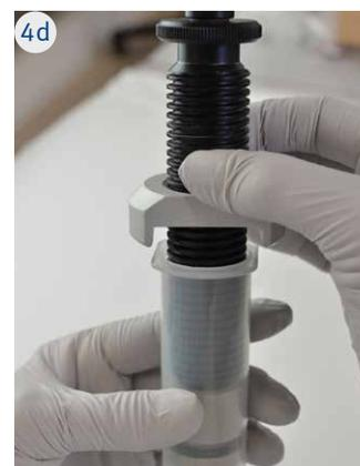
5. Lock the plunger to the cartridge by turning the plunger head until its edges and the edges of the cartridge rim are aligned.
