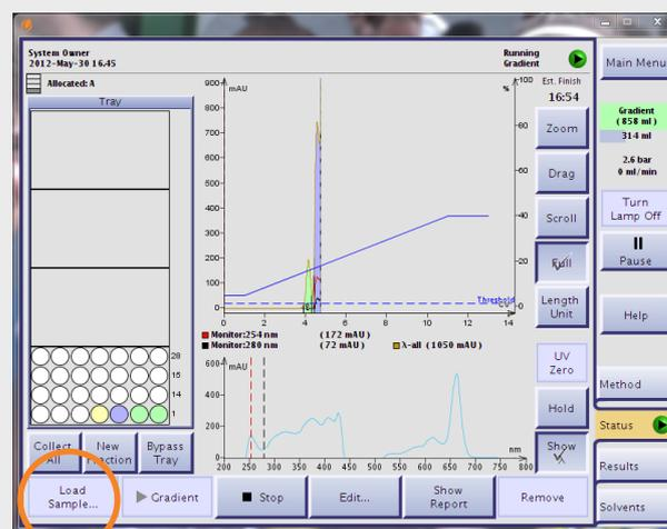
Figure 7. To load, press the "Load Sample" button when using an Isolera system (marked with orange circle).
