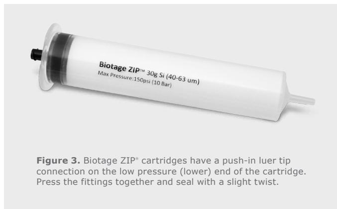
**Figure 3.** Biotage ZIP® cartridges have a push-in luer tip connection on the low pressure (lower) end of the cartridge. Press the fittings together and seal with a slight twist.
