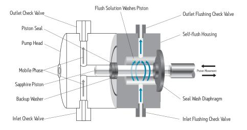
The automatic piston wash improves reliability, extends seal life, and reduces maintenance.
