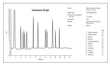
Using Waters Carbamate Analysis System, a smooth baseline and high sensitivity can be achieved for 11 N-methylcarbamate pesticide standards.
