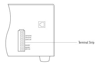
${\it Safe, programmable, unattended operation is possible by means of remote start/stop inputs and a stop output.}$
