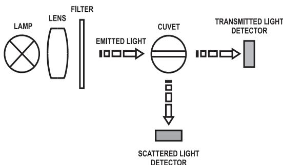
The optical system and measuring technique allow the compensation of lamp intensity fluctuations, minimizing the need of frequent calibration.
