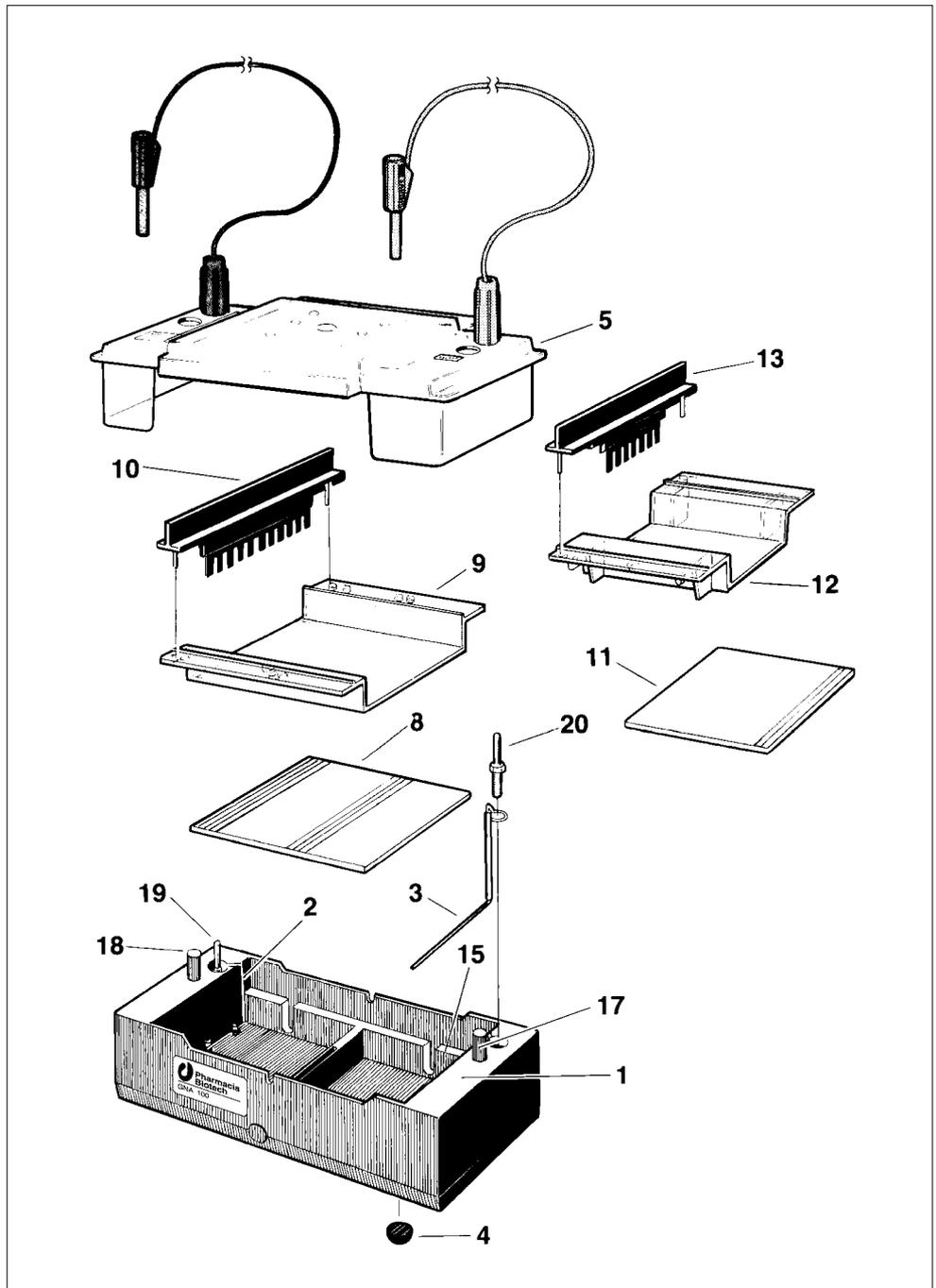
Fig. 4. Exploded diagram of system components.
