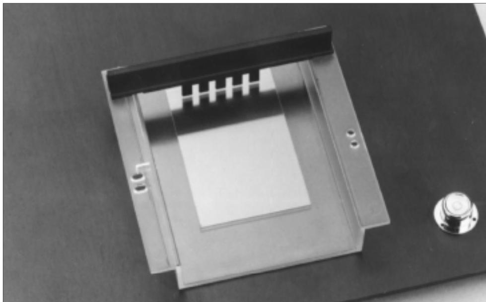
**Fig. 2.** Positioning a glass plate in the gel tray.
