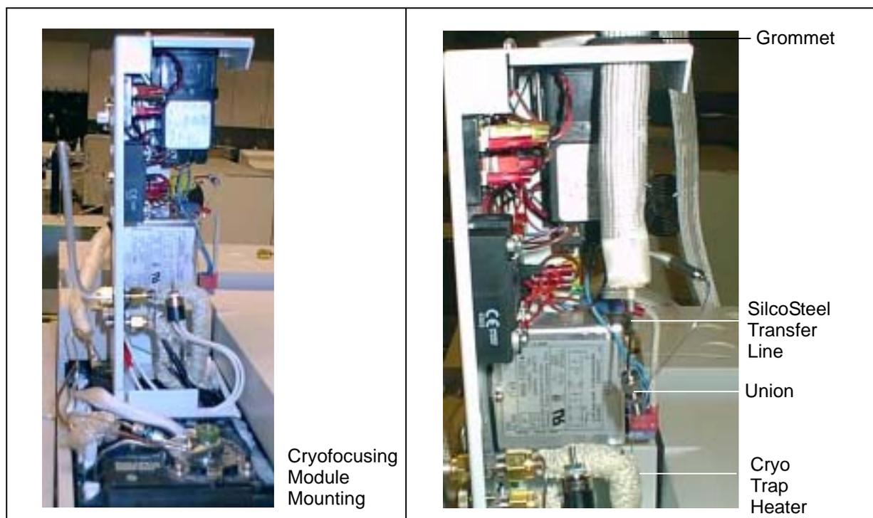
Figure 2-20: Cryofocusing Module Mounted to GC.
