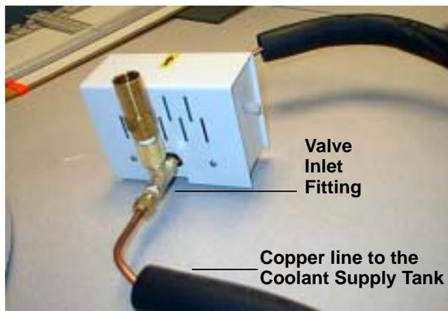
Figure 2-25: Connection from Cryogenic Valve to Coolant Tank
