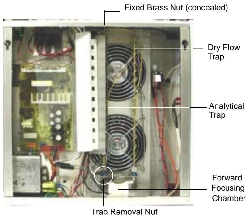
Figure 2-3: Velocity XPT Trap
