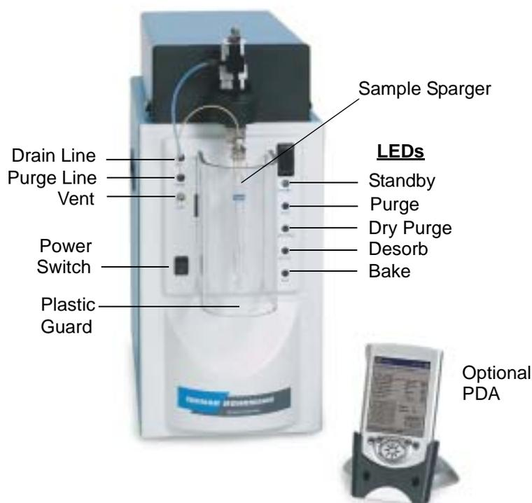
Figure 2-2: Velocity XPT: LEDs, Glassware, and Optional PDA
