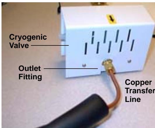
Figure 2-24: Cryogenic Valve: Outlet Fitting
