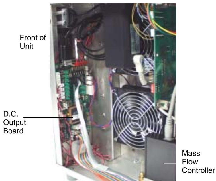
Figure 2-7: D.C. Output Board
