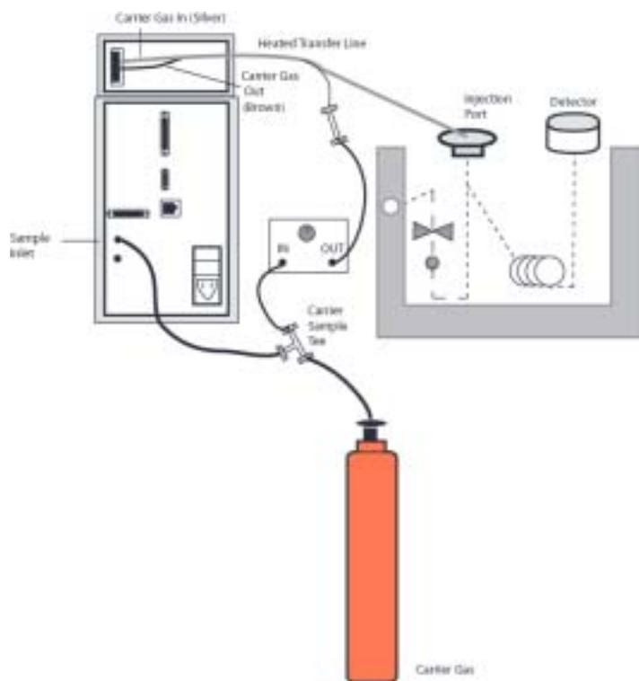
Figure 2-12: Direct Column Connections to the GC
