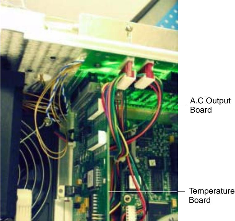
Figure 2-5: Temperature Board
