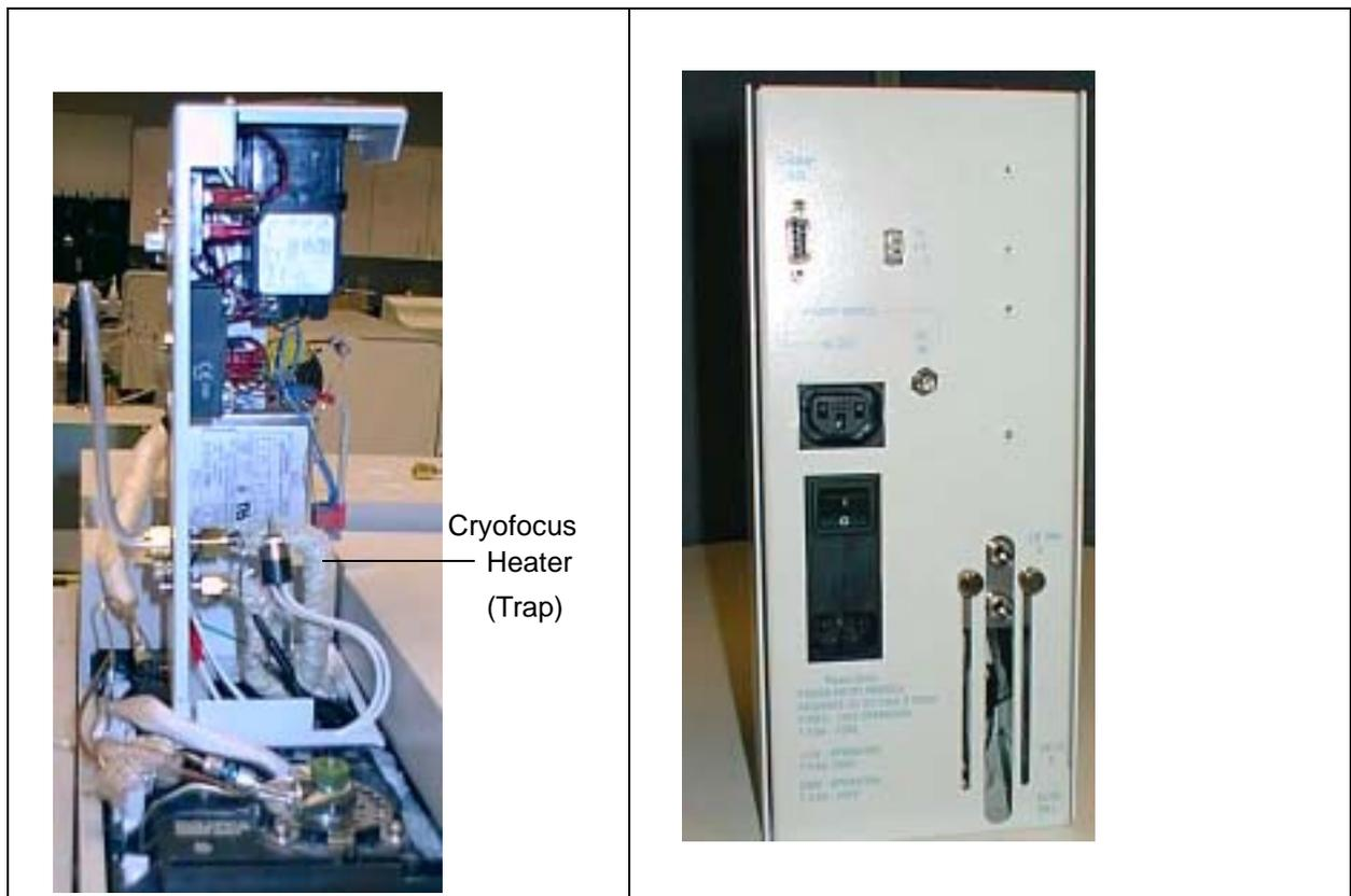
Figure 2-19: Cryofocusing Module (Rear View) and Cutaway View of the Trap
