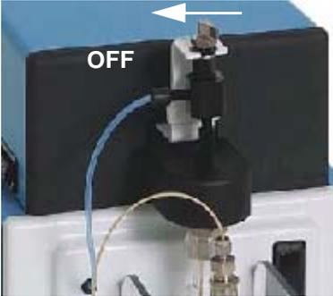
Figure 2-15: Sample Valve Switch
