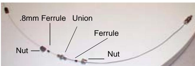
Figure 2-22: Attaching the 1/32" Transfer Line to the GC Column
