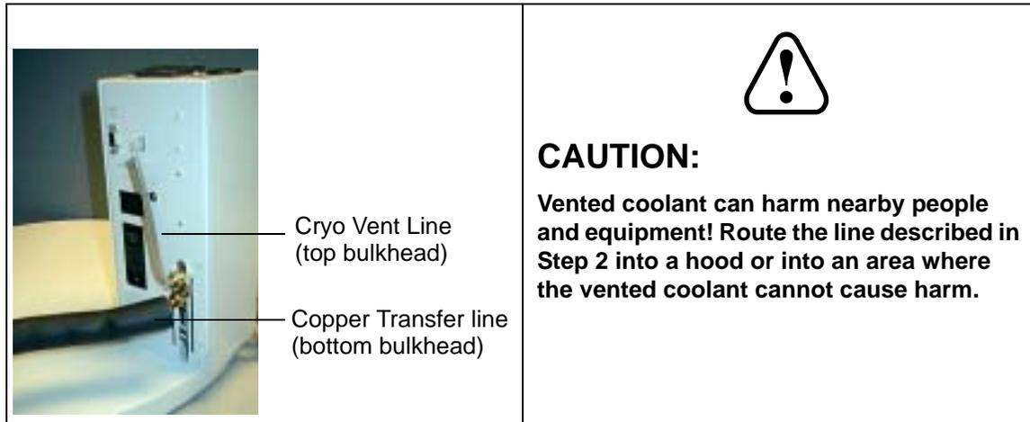
Figure 2-23: Cryo Vent line and Transfer Line Connections
