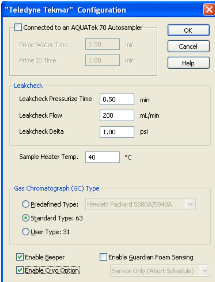
Figure 2-30: Enable Cryo Option
