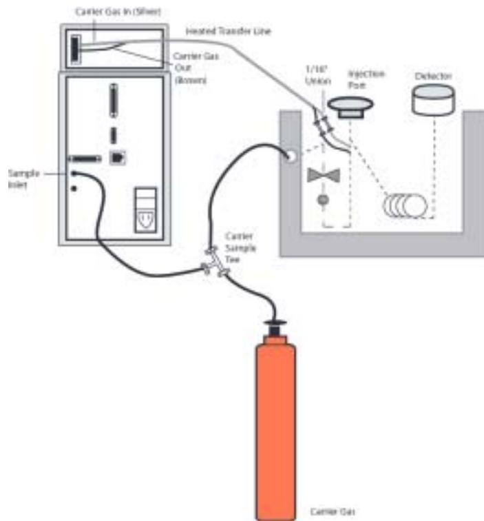
Figure 2-11: Connecting to a Sample Gas Supply
