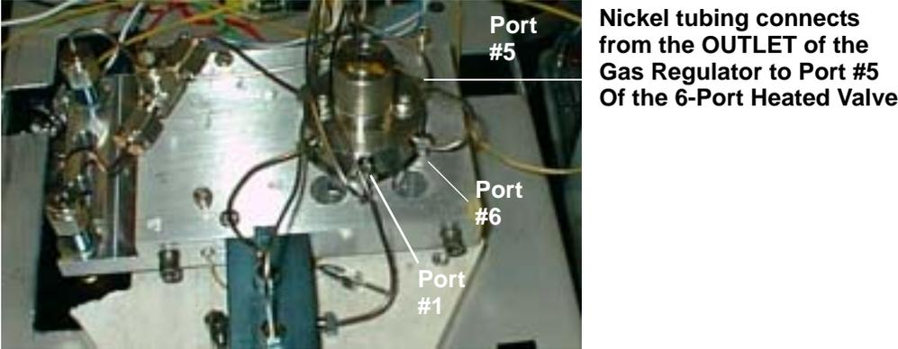
Figure 2-29: Port #5 of the Heated 6-Port Valve
