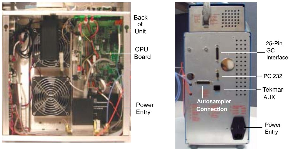
Figure 2-6: CPU Board Connectors
