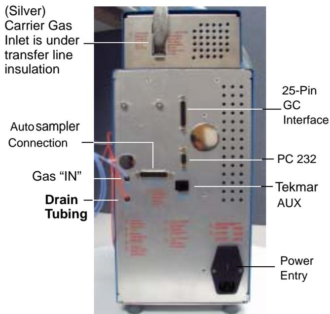
Figure 2-13: Drain Tubing & Electrical Connections
