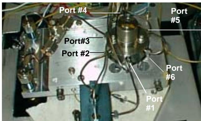
Figure 2-21: 6-Port Valve: Velocity XPT
