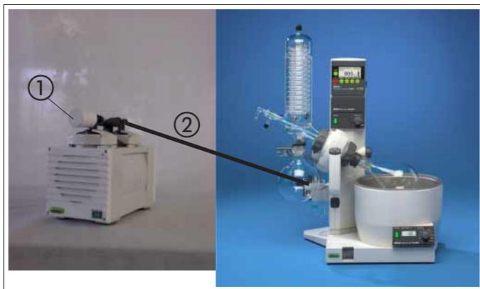
Fig. 15: V-500 connection to Rotavapor
