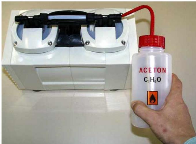
Fig. 24: Cleaning Valve head
