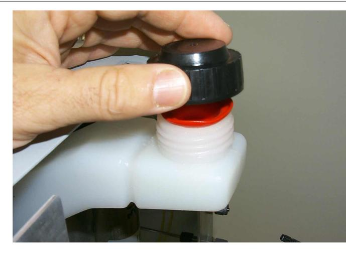
C. Install yellow plug in vent tube and stick label over cap vent as shown
