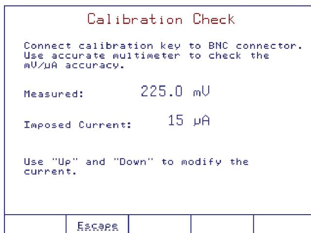
The electrode mV input and the electrode polarization current are measured with the **HI900941** calibration key and a mV/μA multimeter (not included).
