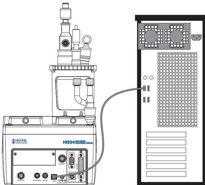
Connect the cable to the USB port on the rear panel of the titrator.
