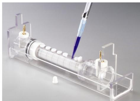
2. Insert the Sample Chamber Caps on the Sample Chambers.
