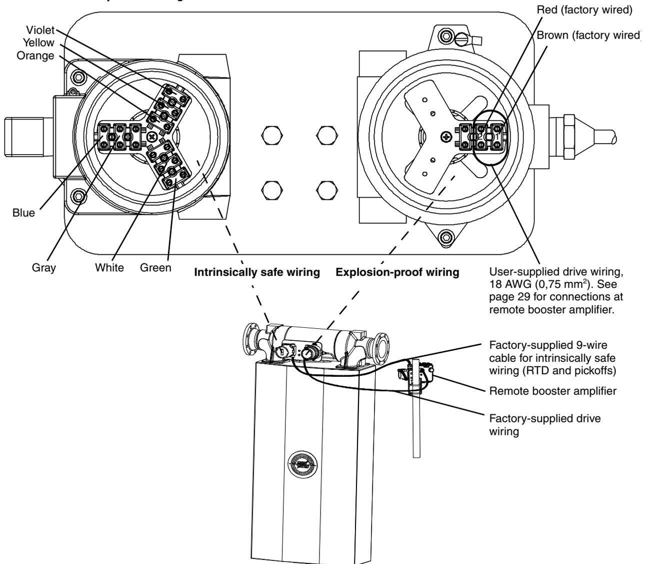
**Remote booster amplifier drive wiring**
