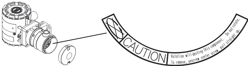
(label inside core processor housing)
