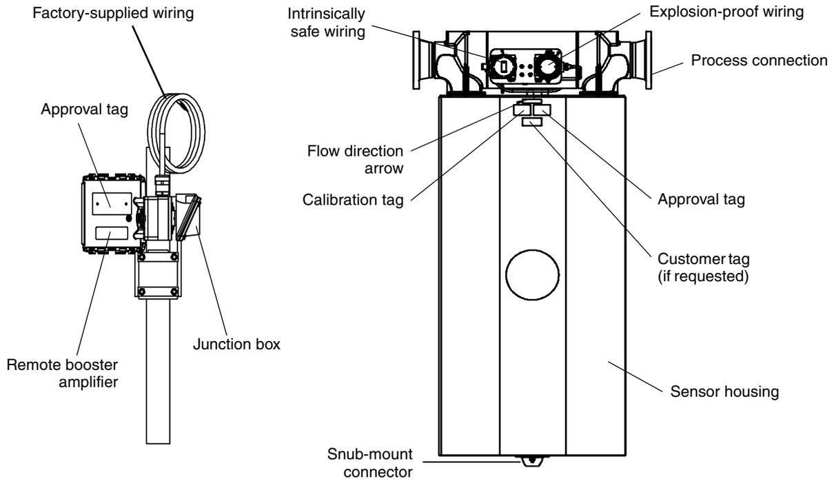
**D600 sensor with remote booster amplifier and core processor**
