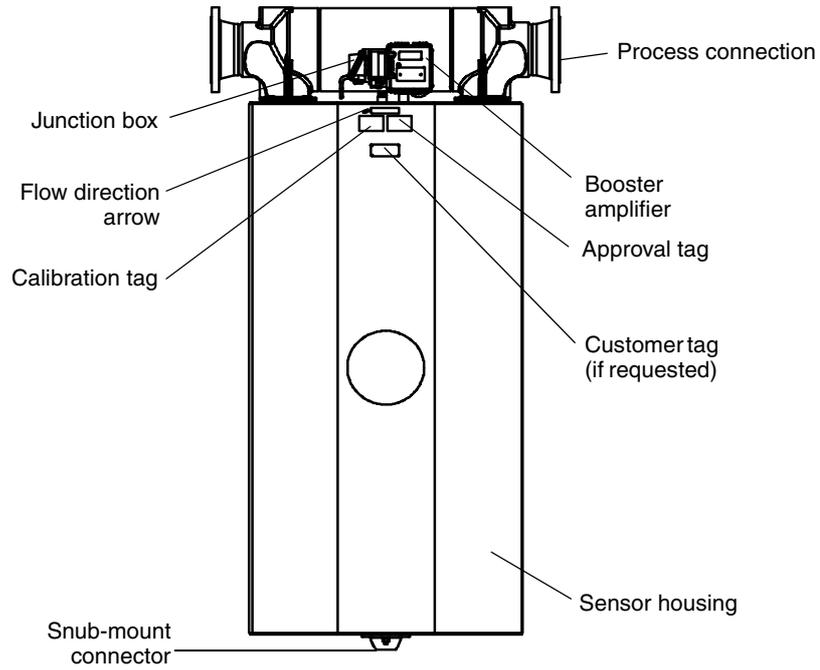
**D600 sensor with integral booster amplifier and core processor**
