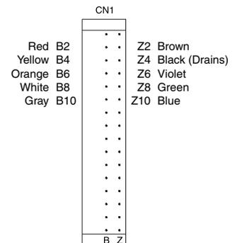
**Model D600 wiring to RFT9712 transmitter**
