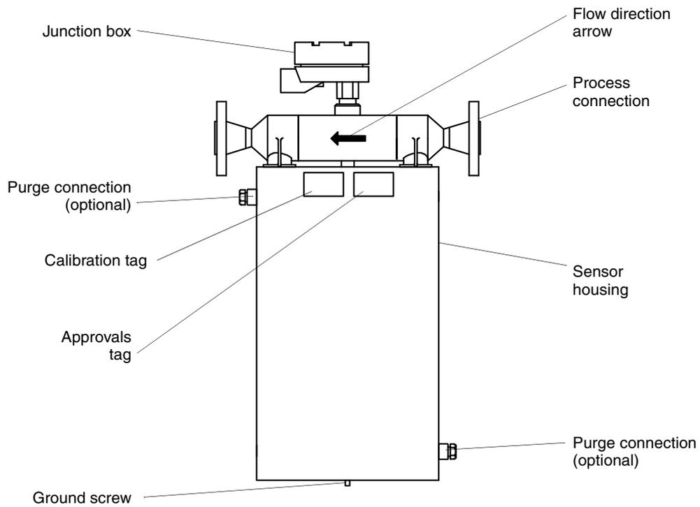
**D600 sensor with integral booster amplifier and junction box**
