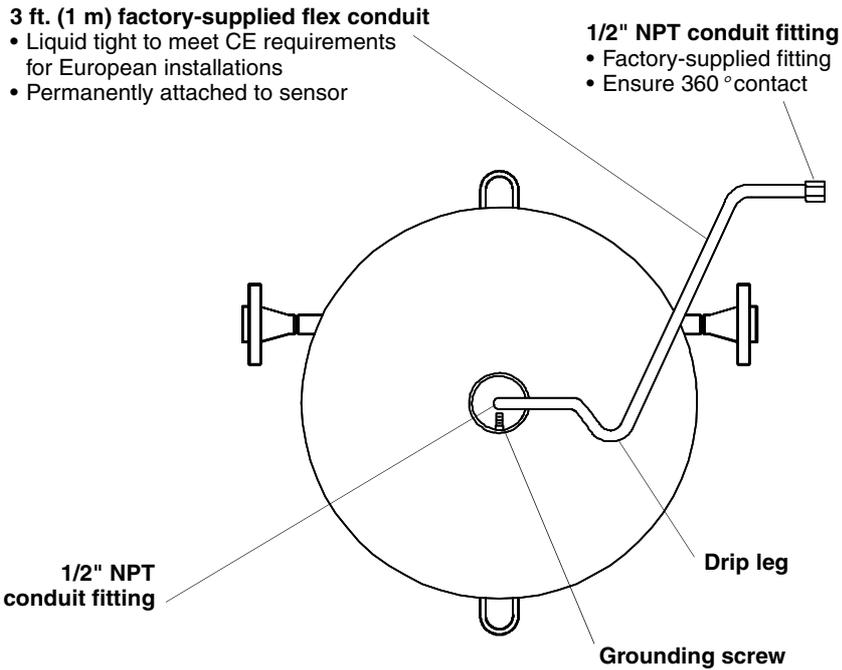
**Connecting and shielding 9-wire cable**
