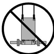
Using the sensor to support piping can damage the sensor or cause measurement error.
