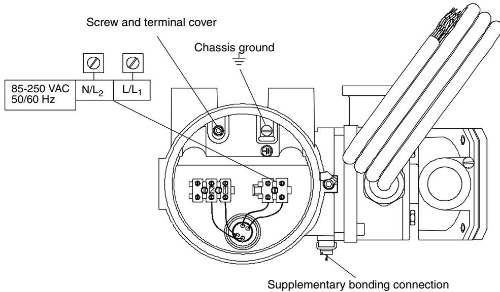
**Power supply wiring to the integral booster amplifier**
