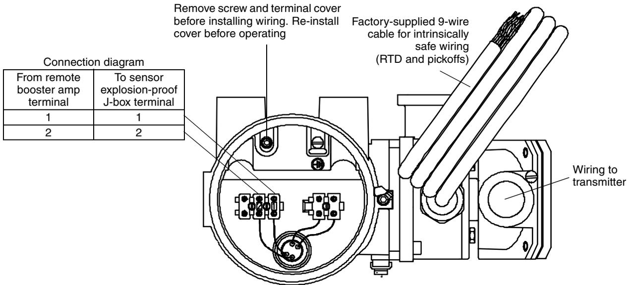
**Wiring to a transmitter (D600 sensor with junction box)**
