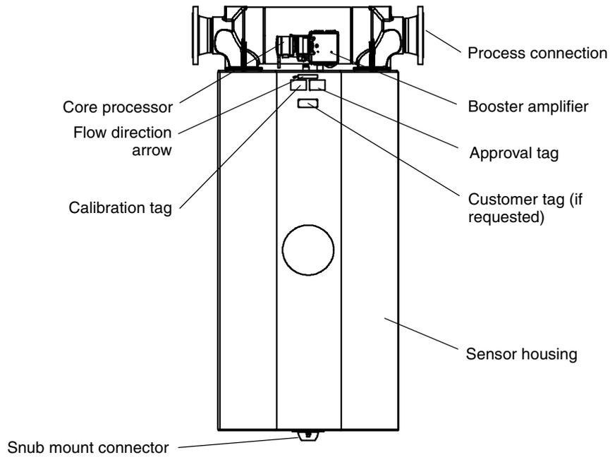
**D600 sensor with remote booster amplifier and junction box**
