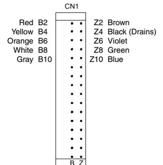
**Model D or DT sensor (except D600) wiring to RFT9712 transmitter**
