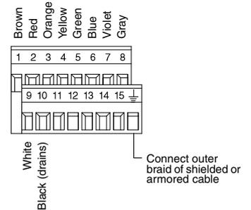
**Model D or DT sensor (except D600) wiring to Model 3500 with screw or solder terminals**
