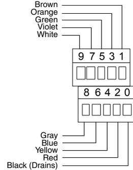
**Model D sensor or DT (except D600) wiring to Model 1700 or 2700 transmitter**
