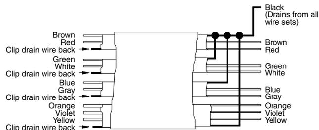
Prepare cable in accordance with the instructions that are shipped with the cable
