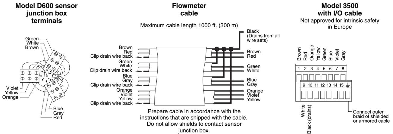
**Model D600 wiring to Model 3500 with screw or solder terminals**
