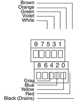
**Model D600 sensor wiring to the 9-wire Model 1700 or 2700 transmitter**
