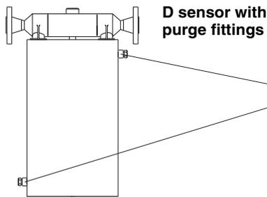
**CAUTION:** Removal of plugs will require sensor case to be repurged with a dry inert gas.
