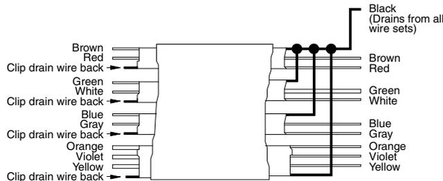
**Model 3500 with screw-type or solder-tail terminals**
