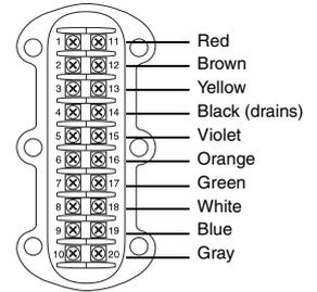
**Model D600 wiring to RFT9739 field-mount transmitter**
