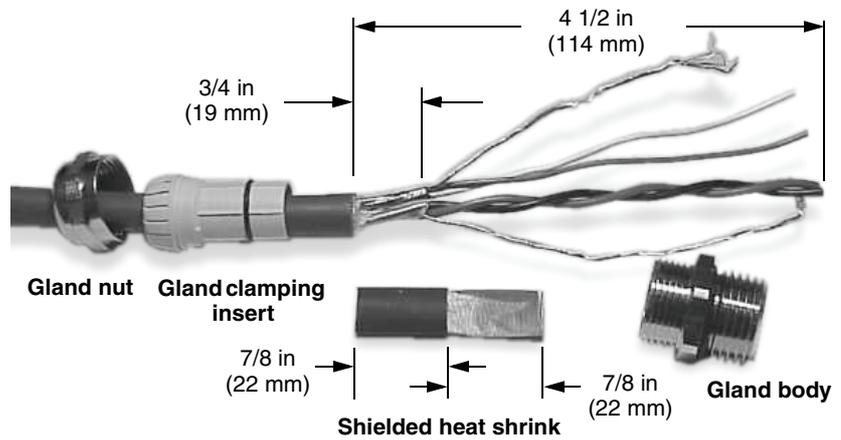
4. For connection at the core processor housing, prepare shielded cable as follows (for armored cable, omit steps d, e, f, and g):
