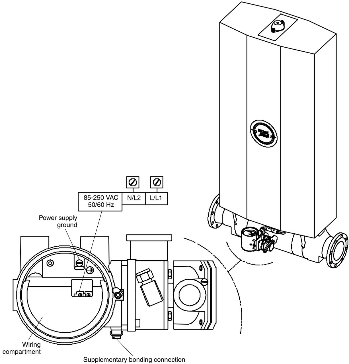
**Wiring from the remote booster amplifier to the sensor**
