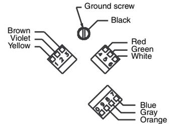
**Model D sensor wiring (except the D600) to IFT9701\* and Model 5300 transmitters**
