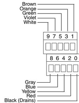
**Model D600 wiring to RFT9739 rack-mount transmitter**
