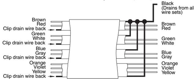
Prepare cable in accordance with the instructions that are shipped with the cable. Do not allow shields to contact sensor junction box.
