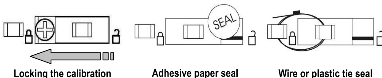
Figure 4-1. Locking and Sealing the Calibration Lock Switch.
