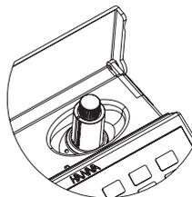
**Note:** Phase separation must be complete before the measurement is taken. If the solution is cloudy, the separation between the organic and aqueous layer can be improved by gently warming the vial (holding the vial in your hand). If the organic layer contains some aqueous drops hanging on the vial wall, gently swirl or invert the vial.
