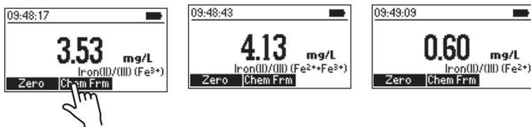
**Note:** Each chemical form can be logged independently by pressing the **LOG** key.
