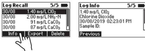
Use **Delete** to erase logged data. After pressing **Delete** the prompt on the display will confirm the action.
