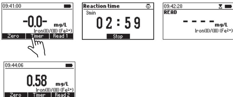
*Warning: Timing is critical for accurate measurement. Reaction times beyond 3 minutes may cause some ferric iron (Fe<sup>3+</sup>) to also react, producing false high measurements.*
