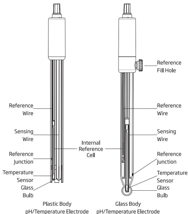
Remove the protective cap. Do not be alarmed if salt deposits are present, this is normal. Rinse the probe with water.
