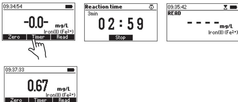
**Warning:** *Timing is critical for accurate measurement. Reaction times beyond 3 minutes may cause some ferric iron ( $\text{Fe}^{3+}$ ) to also react, producing false high measurements.*
