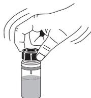
In order to avoid reagent leaking and to obtain more accurate measurements, close the cuvette first with the supplied High-Density Polyethylene (HDPE) plastic stopper
