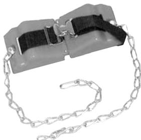
Molded from reinforced polypropylene, the G 110 bracket can be adjusted to snugly support any cylinder from 4.0 to 14.0 inch diameter. Unit is first set to designated cylinder diameter with recessed set screws locking in width position. Permanently mounts to wall using fasteners. Fastener type depends on mounting surface (fasteners supplied by customer). Strap and security chain sets included.
