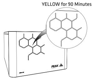
The generator will purge impurities from its internal storage tank until Oxygen content is less than 5PPM, approximately 1.5 hours (3-3.5 hours for Headspace) of uninterrupted operation. On completion, the Fascia will illuminate **GREEN** or **BLUE (70-\*\*\*\* Part Numbers Only)** and the generator is now ready to be connected to the application.
